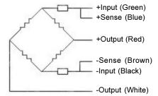
The two "sense" wires sample the bridge supply voltage at the load cell. Complete compensation of change in the lead wore resistance, due to temperature change and/or cable extension, is achieved by feeding this voltage into appropriate electronics.
